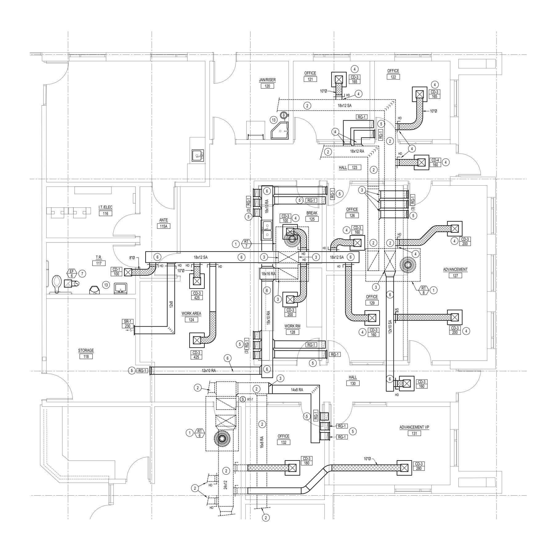
MECHANICAL FLOOR PLAN SCALE: 1/4" = 1'-0" (ALTERNATE #2 BID CONDITIONS.)
